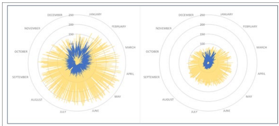
Figure 1. Annual chart reporting hourly building energy use (blue) versus photovoltaic power production (yellow). Baseline building (Left), Passive Building (right). The super-efficient Passive Building on the right needs less solar PV to offset the building energy use than the Baseline Building on the left. (Source: White, 2020)
